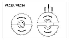
• VRC30 (2 parts) - 30 mm shaft, on the propeller shaft.
